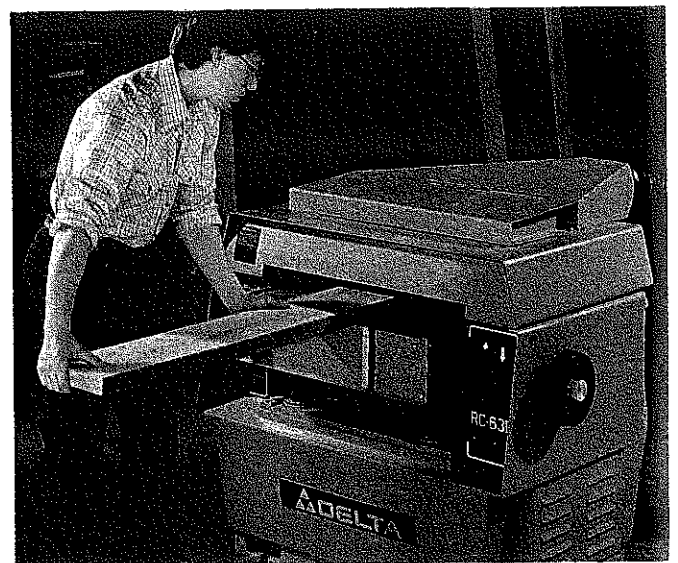
Fig. 10-12. Stand to the side of the stock as you feed it into the planer. (Delta International Machinery Corp.)
